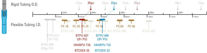
Values are approximate; in particular IDs and ODs of extruded tubing can vary by ±.002in (.05mm) from nominal values. If dead volume is critical measure it directly by comparing weights of filled and empty samples.
