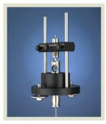
This heavy-duty swivel holder bolts to the top of the cage and allows all of Instech's single and dual channel swivels to be used with dogs, nonhuman primates and other large animals. For cleaning, simply remove the swivel and the stainless steel posts and send the rest of it through a cage washer with the cage. The mount couples directly to standard <sup>1</sup>/<sub>2</sub>-in (12.7mm) ID jacket tethers.
