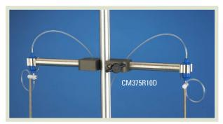
This swivel holder mounts to poles that are 3/8 to 1/2-inch (9-12mm) in diameter. It features a clip that allows for easy snap-in, snap-out installation and removal of an Instech swivel. The clip can rotate in one axis as the animal moves and includes a stop to prevent the swivel from slipping downward. The distance from the mounting pole to the swivel is approximately 10cm. Available in single- and double-sided versions.
