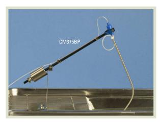
This mount is designed for standard infusion of rats in shoebox cages. The mount pivots in the vertical plane to remove slack from the tether but allow enough length to reach all corners of an asymmetrical cage. The adjustable counter-weight can be set to balance the weight of our swivels plus a tether. The crossbar in the wire top must be clipped in the slot that the tether is placed for maximum travel.
